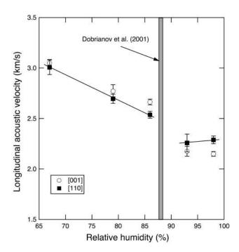
FIGURE 4 Sound velocity of tetragonal lysozyme along the [110] and [001] directions as a function of RH. There is a discontinuous increase of both velocities and an inversion of the velocity ratio in the 93%–87% RH range.
