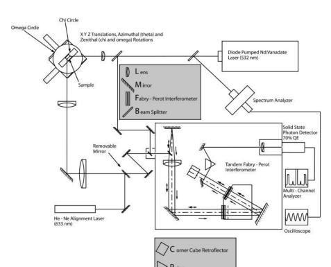
FIGURE 2 Schematic diagram of the Brillouin scattering system.
