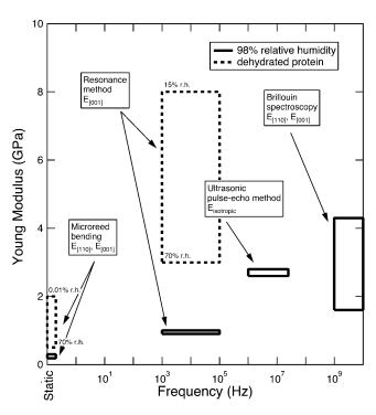
FIGURE 7 Range of values of the Young's moduli of tetragonal lysozyme crystals as determined using different techniques in different frequency ranges. See Table 1 for the data references.
