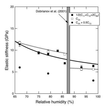
FIGURE 5 Elastic constant  $C_{33}$ , and the combinations  $\frac{1}{2}(C_{11} + C_{12} + 2C_{66})$  and  $C_{44} + 0.5C_{13}$  (see text) of tetragonal lysozyme crystals plotted as a function of RH. The solid line is the best fit to the structural model for  $\frac{1}{2}(C_{11} + C_{12} + 2C_{66})$ , whereas the dashed line is the best fit for  $C_{33}$ .
