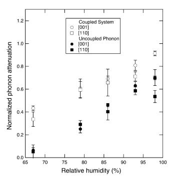
FIGURE 8 Normalized phonon attenuation  $\alpha \lambda_S$  as a function of RH, calculated for phonons propagating along the [110] and [001] directions. Both coupled and uncoupled values are shown for comparison.
